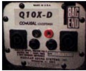
Input options galore: A rear-mounted jack panel houses two parallel 1/4” jacks, two parallel Neutrik Speakon connectors, and one banana-jack input.
