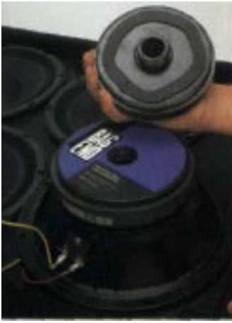
The E-550 titanium compression high-frequency driver module screws into the rear of the E-10X low frequency driver.
