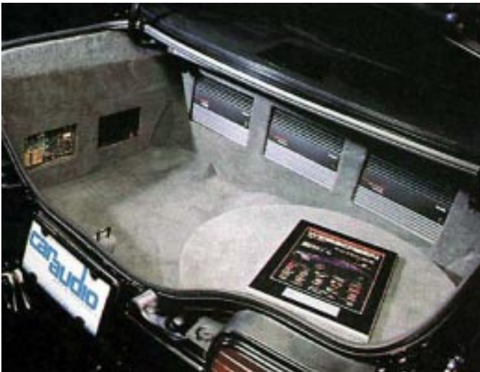
With the trunk open, the system components are exposed. The system includes three Coustic amplifiers for the LF, RF, LS, RS, and both subwoofer channels. The DTS and Circle Sound processors are visible on the driver's side of the trunk.
