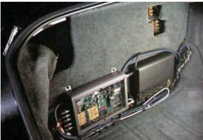
More detail comes into view as the final trim panel is removed, exposing the two surround-sound processors and the center-channel amplifier.
