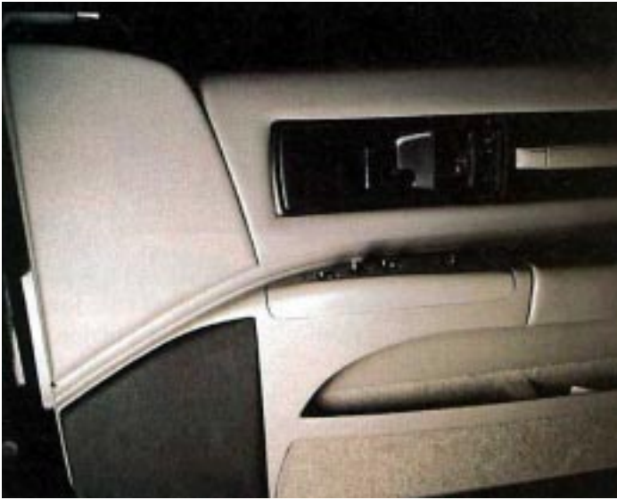
The front door panels and structures (above) were modified to replace the stock 6-inch factory speakers.
