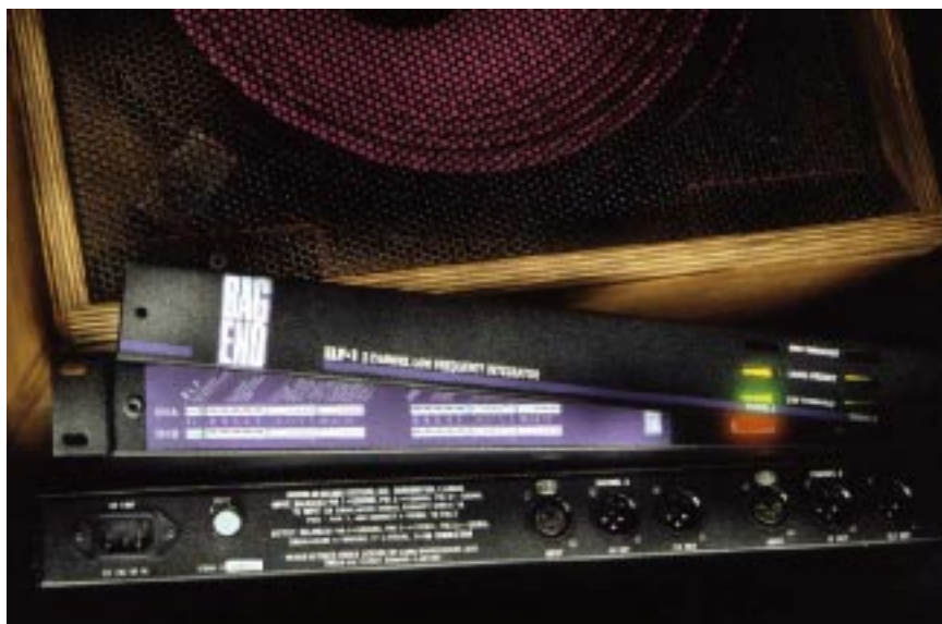
FIG 1: The 90 DIP switches hidden behind the front panel of Bag End's ELF-1 2-channel Low Frequency Integrator are used to configure both the highpass filter and the ELF. The switches add precision resistors whose value establishes a DC voltage that controls the appropriate circuits inside the unit.
